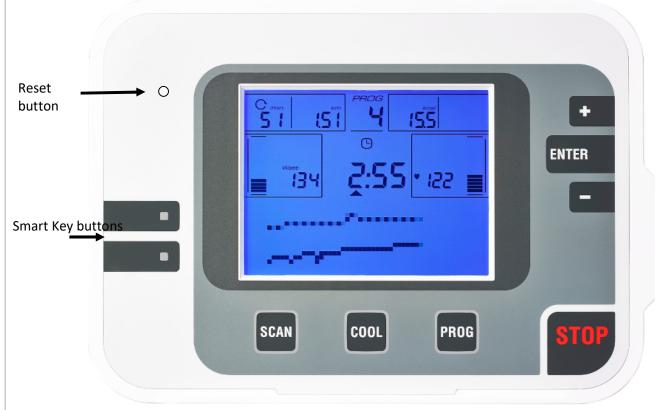
Fig. 2: Monitor view for explanation of button functions
